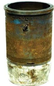
**Inhibitors:** There are two general categories of inhibitors: inorganic and organic. Organic acid technology (OAT) inhibitors are preferred by today's original equipment manufacturers (OEMs) and eliminate the need to add or maintain supplemental coolant additives (SCAs). OAT inhibitors are opportunistic by moving to trouble spots as needed and selectively protect the cooling system, resulting in longer-lasting protection.
