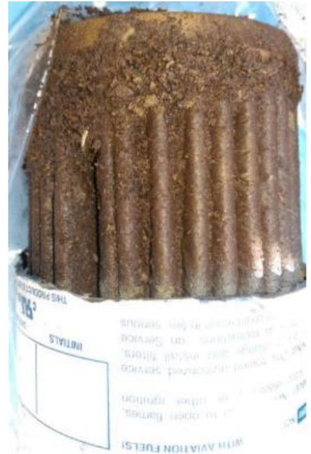
Filter plugged with fuel tank sediment
